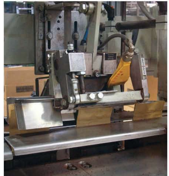
TRIMMING WASTE. The Corner Seal bag trimmer trims extra film from the coffee pouch. Peerless has modified this component and film measurements to minimize waste.
